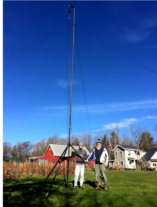
John Colt, NV1Y, and Leandra MacLennan, AR1R Mast for Off-center fed wire dipole.
